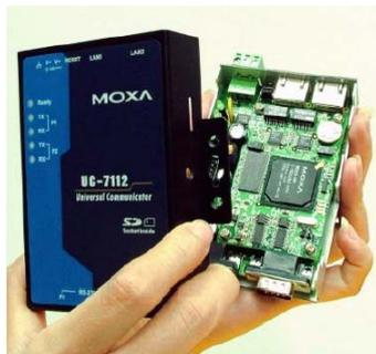
**Step 3:** The SD socket is located on the back of bottom board. Insert the SD memory card as shown in the figure.
