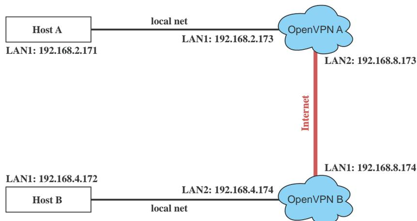
Host A (B) represents one of the machines that belongs to OpenVPN A (B). The two remote subnets are configured for a different range of IP addresses. When this setup is moved to a public network, the external interfaces of the OpenVPN machines should be configured for static IPs, or connect to another device (such as a firewall or DSL box) first.
