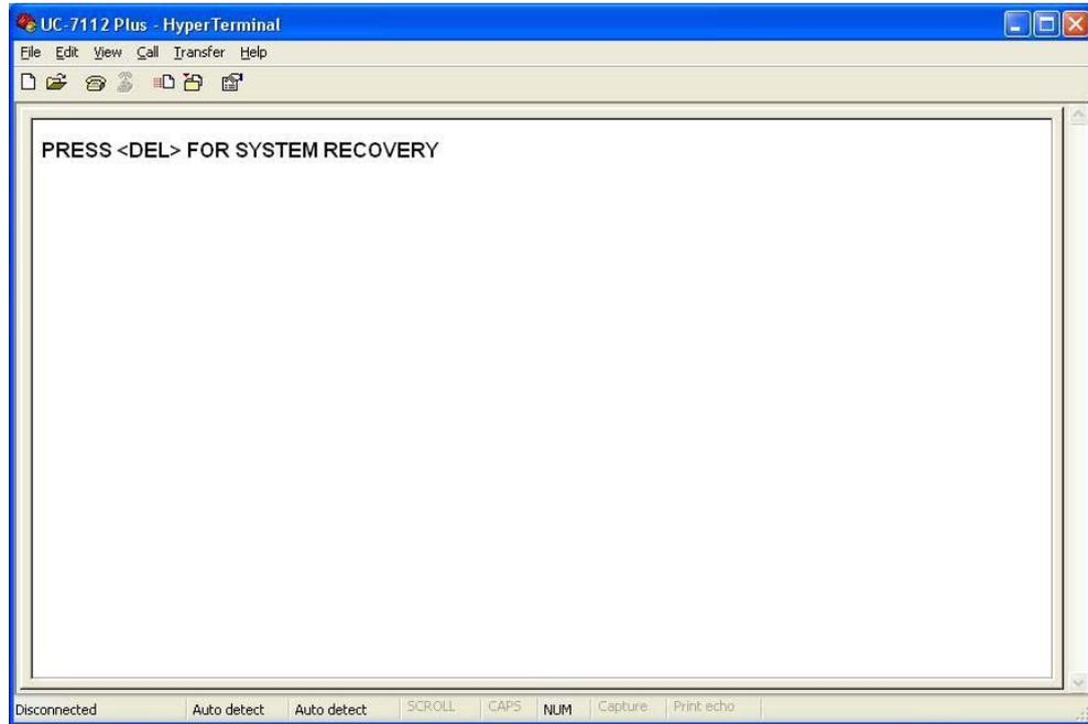
2. Some models support the boot loader utility, but the screen will not appear. In this case, hold down the **DEL** key on your PC and then power on the embedded computer again. If the boot loader utility menu appears, continue to the next chapter for firmware upgrade or recovery instructions.
