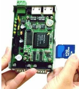
**NOTE:** To remove the SD card from the slot, press the SD card in slightly with your finger, and then remove your finger to cause the card to spring out partially. You may now grasp the top of the card with two fingers and pull it out.
