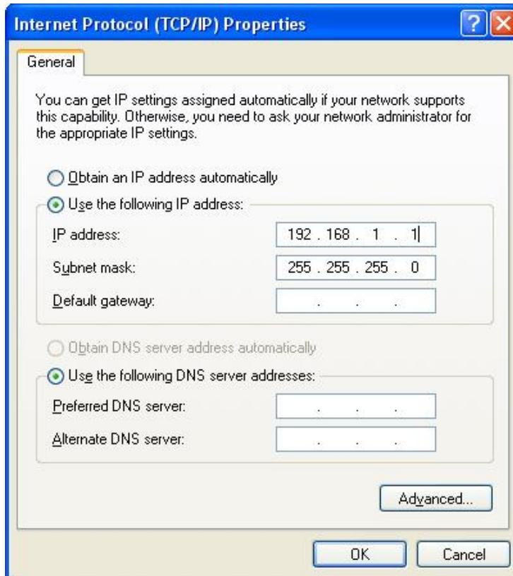
8. Go back to the boot load utility menu and enter the local IP address. This local IP address is the IP address of the embedded computer. **Note that the local IP address must be on the same network as the server IP address.** For example, if the server IP address is 192.168.1.1, you can choose a local IP address from the range 192.168.1.2 to 192.168.1.255.
