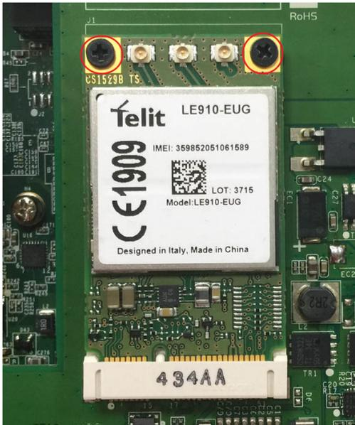
3. Attach one end of the cellular cable on the central connector, and then connect the other end of the cable on the W1 hole on the front panel of the computer. Remove the antenna hole protection cover before you do so.
