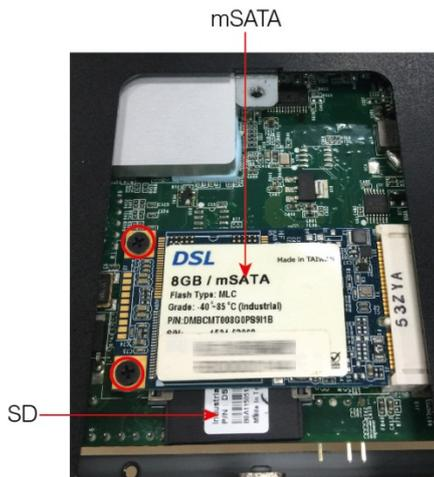
3. Push the SD card in gently to release it and remove the SD card to insert a new one in the socket. Please note that the SD card comes with a pre-installed operating system. For details on Operating System recovery, refer to the UC-8410A User's Manual.
