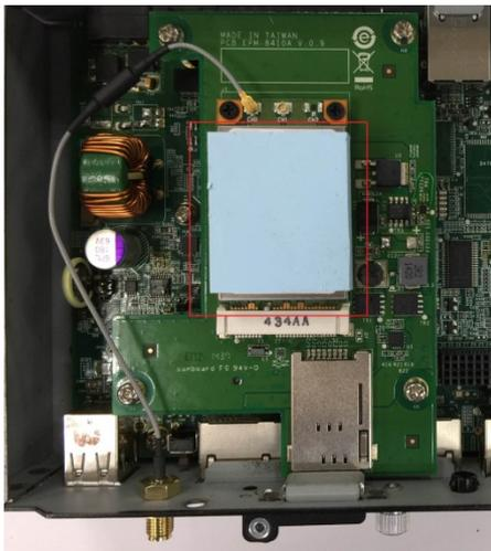
6. Connect the Wi-Fi antenna to the computer via the connector provided on the rear panel.
