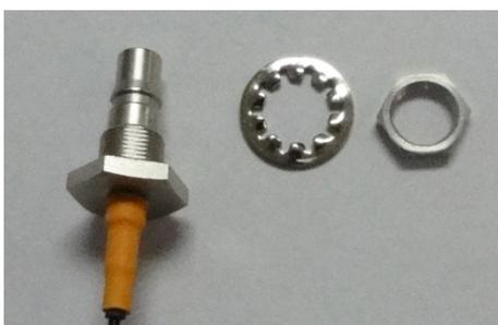
7. Pass the antenna mount's threaded connection ring through the mounting hole; keeping the locking washer against the rear panel face, secure the antenna connector by by tightening the provided nut onto the threaded protection ring.
