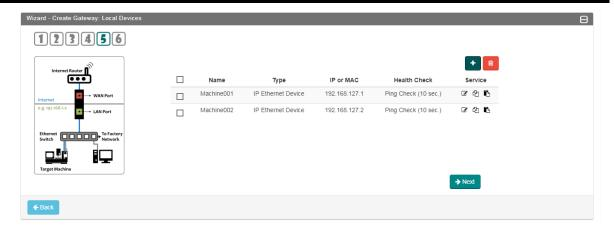
Click of to edit the available service of the device for remote access. By default, the remote access function can connect to all the services of the device. To enhance security, you can limit each of the services to selected MRC clients only.
