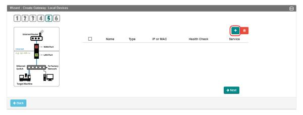
In put the local device name and the local original IP address of the target Ethernet devices or machines. If the local Ethernet device is a layer 2 device, please input the device's MAC address. The gateway can also perform a health check of the connection through Ping Check or Port Link. (If a switch is connected to the gateway's LAN port, Ping Check is recommended. If a machine is directly connected to the gateway, Port Link is also an option.)
