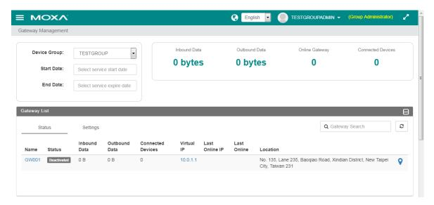
In the middle of the page, the group administrator can monitor the status for all the individual gateways in the device group including the data usage, the connected devices, and the gateway's virtual IP address.
