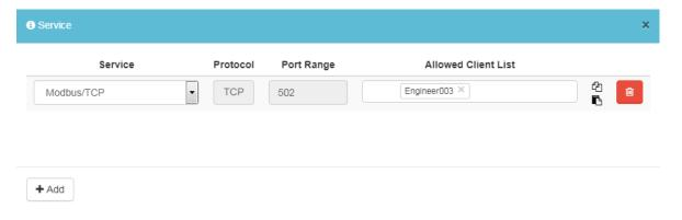
**NOTE** For site-to-site networking, leaving the device list empty allows a remote connection to access the WHOLE LOCAL SUBNET defined as the LAN subnet of the gateway. For example, if the LAN configuration of the gateway is 192.168.127.254/24, all the Ethernet devices or machines with the IP address 192.168.127.x connected together with the MRC gateway's LAN are available for remote access.
