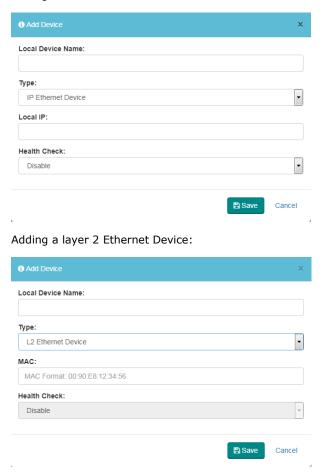
**NOTE** In order to enhance cyber security, remote access will be limited to defined Ethernet devices in the MRC gateway and does not interrupt or disrupt the original factory network. A maximum of 25 devices can be added into the list for remote access.
