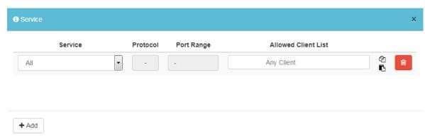
For example, there is a Modbus TCP device that only allows Engineer003 to have remote access. You can configure the service to the MRC client as shown below. Multiple service rules are acceptable for a service whitelist.
