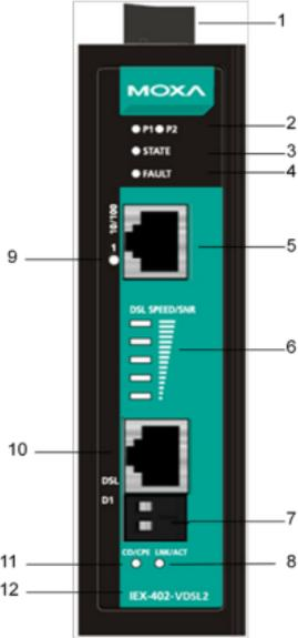
1. Terminal block for power input (PWR1, PWR2)
