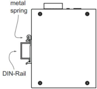
To remove the Moxa Ethernet Extender from the DIN rail, simply reverse steps 1 and 2.
