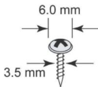
**NOTE** Before tightening the screws into the wall, make sure the screw head and shank size are suitable by inserting the screw into one of the keyhole-shaped apertures of the wall mounting plates.
