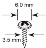
Do not drive the screws in all the way—leave a space of about 2 mm to allow room for sliding the wall mount panel between the wall and the screws.
