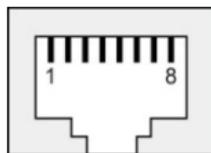
**NOTE** The pin numbers for both 8-pin and 10-pin RJ45 connectors (and ports) are typically not labeled on the connector (or port). Refer to the pinout diagram above for details.
