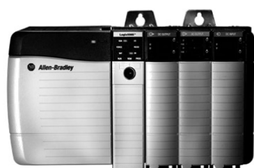
Allen-Bradley PLC IP: 192.168.108.200
