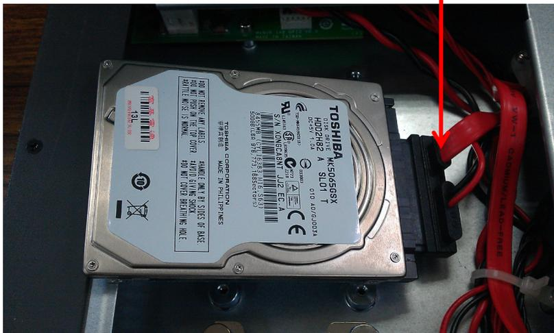
**Step 5:** Place the hard drive disk on the bracket, and then use the 4 HDD screws to fasten it.
