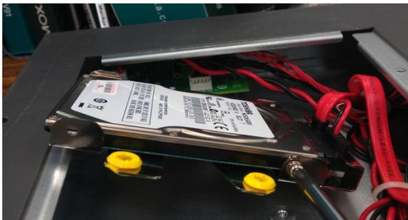
**Step 6:** Fasten the 4 bracket screws
