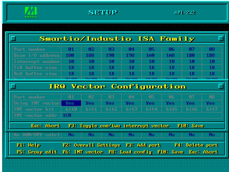
4. Press **F10** to save the latest configuration and exit the SETUP program.
