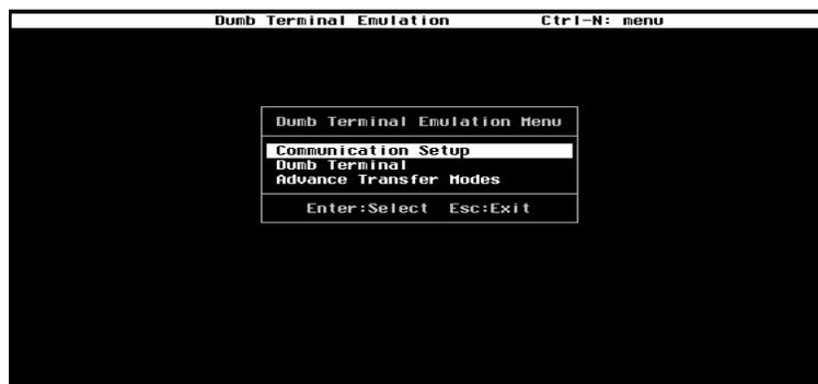
1. Select and Press Enter on item “**Communication Setup**” to setup up all the communication parameters for connection.
