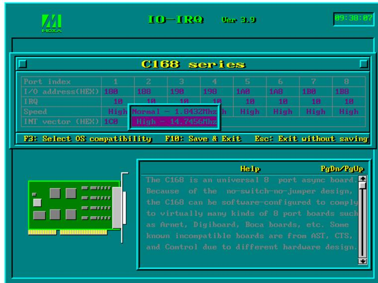
Note that, currently, port that uses **MOXA Windows NT and 95/98 driver** will run at the displayed speed. To be clear, when Smartio C168 Series board is configured as **High Speed Spectrum**, any port driven by the **Moxa-provided Windows NT and 95/98 driver** will display the exact working speed. For example, the displayed speed 38.4 Kbps is equal to the working speed 38.4 Kbps.
