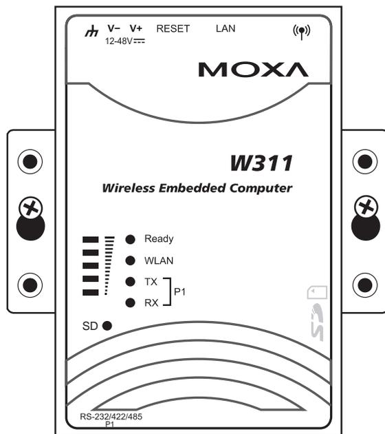
For the W341, it comes with two metal attachment plates for attaching the embedded computer to a wall or the inside of a cabinet. First, use two screws per bracket to attach the brackets to the rear of the W341. Next, use two screws per bracket to attach the W341 to a wall or cabinet.
