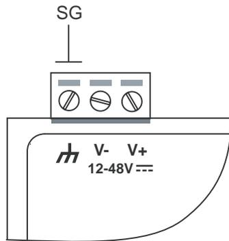
**SG:** The *Shielded Ground* (sometimes called Protected Ground) contact is the left most contact of the 3-pin power terminal block connector, as viewed from the angle shown here. Connect the SG wire to an appropriate grounded metal surface.
