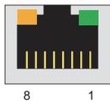
The LED indicator on the right glows a solid green color when the cable is properly connected to a 100 Mbps Ethernet network. The LED will flash on and off when Ethernet packets are being transmitted or received.
