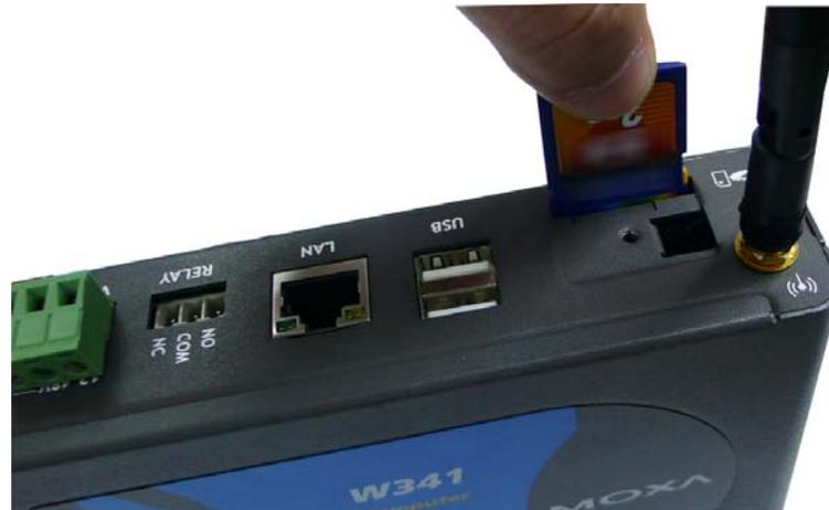
**NOTE:** To remove the SD card from the slot, press the SD card in slightly with your finger, and then remove your finger to cause the card to spring out partially. You may now grasp the top of the card with two fingers and pull it out.
