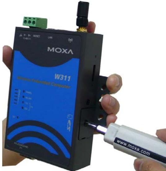
Step 2: After removing the cover, insert the SD memory card as shown.
