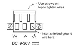
**SG:** The Shielded Ground (sometimes called Protected Ground) contact is the right most contact of the 3-pin power terminal block connector, as viewed from the angle shown here. Connect the SG wire to an appropriate grounded metal surface.
