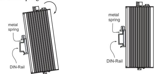
To remove V481 from the DIN-Rail, simply reverse Steps 1 and 2.
