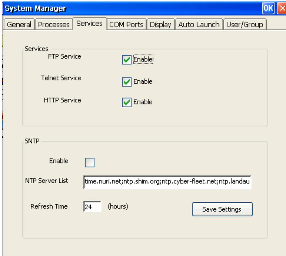
You can also use SNTP to synchronize the system time. To do this, click the enable check box under SNTP, and then type the NTP server list in the text field and enter a refresh time. Click “Save Settings” after you finish the configuration.
