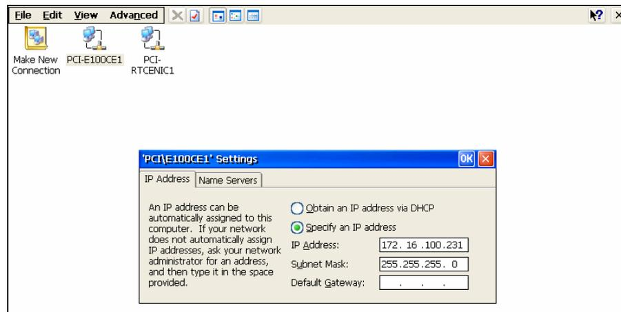
**Step3:** Input the new IP address and netmask and then click **OK**.
