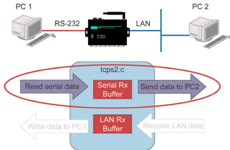
**NOTE** The `tcps2.c` application is a simple example designed to give users a basic understanding of the concepts involved in combining Ethernet communication and serial port communication. However, the example program has some limitations that make it unsuitable for real-life applications.
