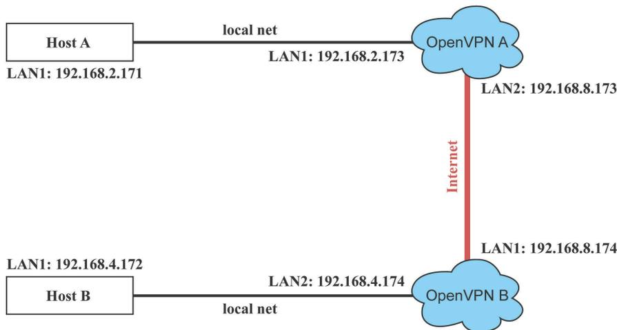
2. The configuration procedure is almost the same as for the previous example. The only difference is that you will need to comment out the parameter "up" in "/etc/openvpn/A-tap0-br.conf" and "/etc/openvpn/B-tap0-br.conf".
