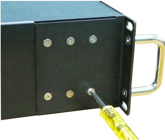
**Step 4: Installing the DA-682 to a rack.**
