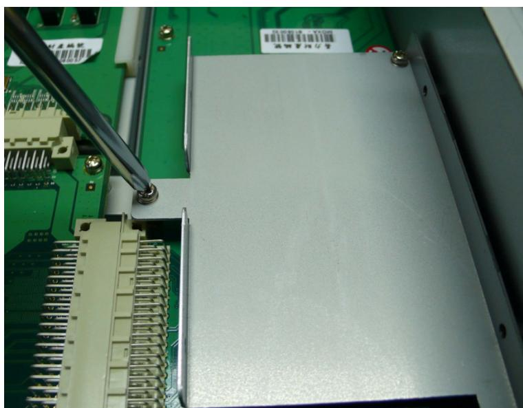
4. Install the SATA hard disk in the hard disk bracket.
