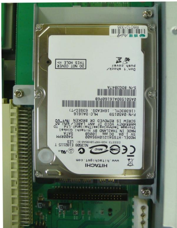
6. Connect the SATA disk cable and power cable to the SATA hard disk.
