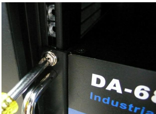
As a final check, make sure that the four screws are firmly attached to the rack.
