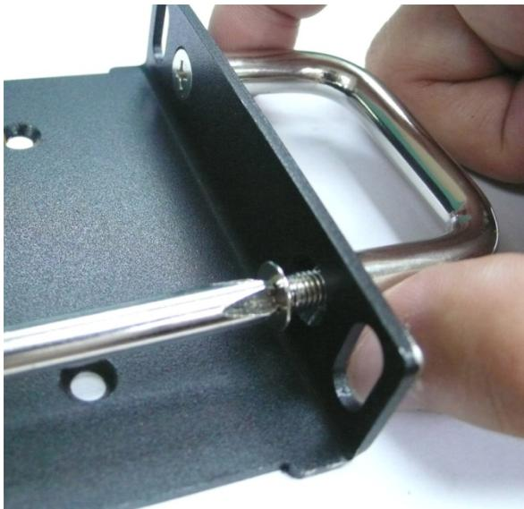
**Step 3: Installing the rackmount ears to the DA-682.**
