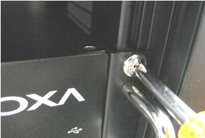
Note that four screws are required to attach the DA-682 to the rack. Use two screws on the left side and two screws on the right side.
