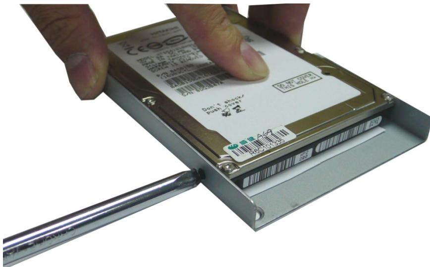
5. Next, install the SATA hard disk and hard disk bracket back into the DA-682.
