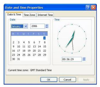
Go to **Date/Time properties** → **Intenet Time** to adjust the NTP server setting.
