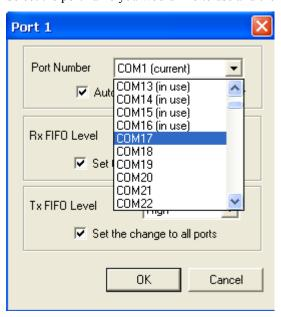
MOXA MU860 UART CHIP (PCI Bus) Properties General Ports Configuration Driver Details Resources Port COM No. Rx FIFO Level Tx FIFO Level High, **COM 17** 2 3 **COM 18** High High COM 19 High High 4 COM 20 High High 5 COM 21 High High 6 COM 22 High High Help COM 23 High High 8 COM 24 High High Port Info Port Setting
