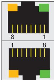
The LED indicators on the right top and right bottom corners glow a solid green color when the cable is properly connected to a 100 Mbps Ethernet network. The LED will flash on and off when Ethernet packets are being transmitted or received.
