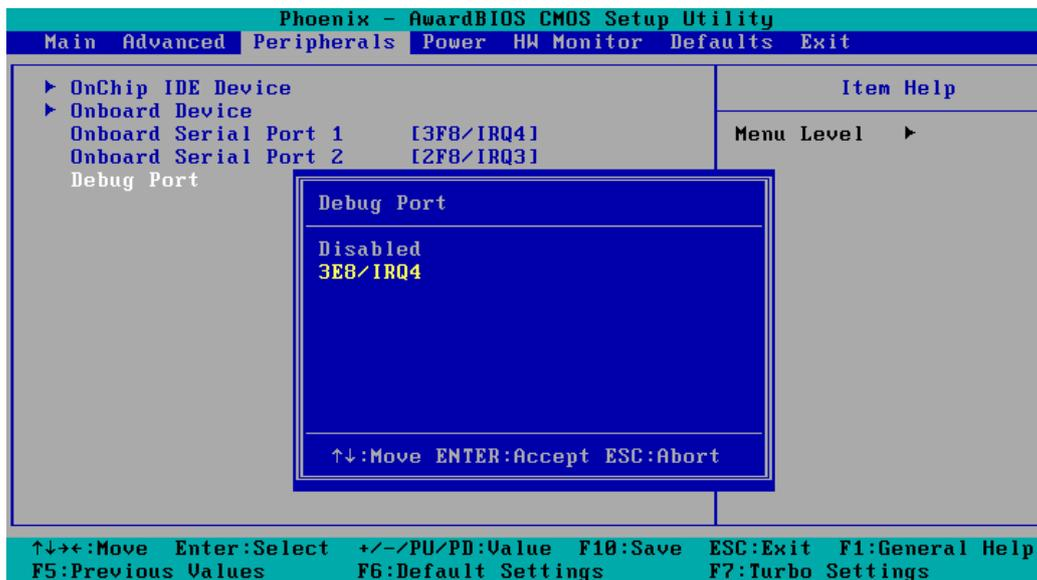
This function allows you to enable/disable the debug port communication. The V2101 computer will automatically distribute the IRQ value for the debug port as the default value. If you wish to disable, select **Disabled**. This port is only for engineers who are debugging programs.
