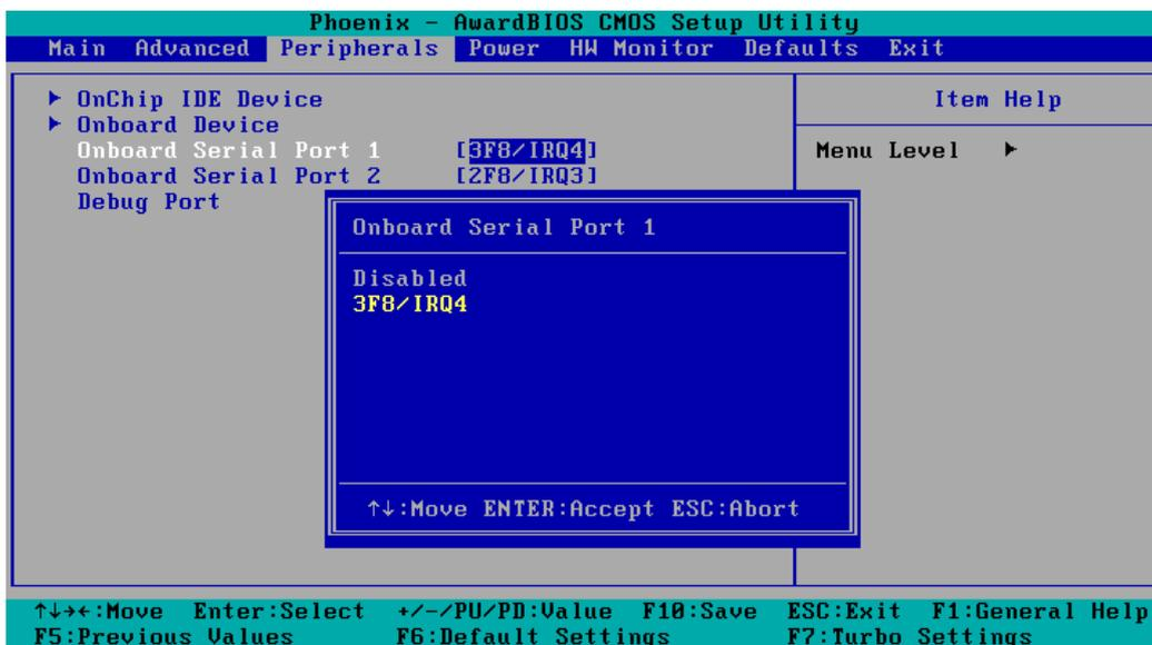
This function allows you to enable/disable serial port 1 communication. The V2101 computer will automatically distribute the IRQ value for serial port 1 as the default value. If you wish to disable, select **Disabled**.
