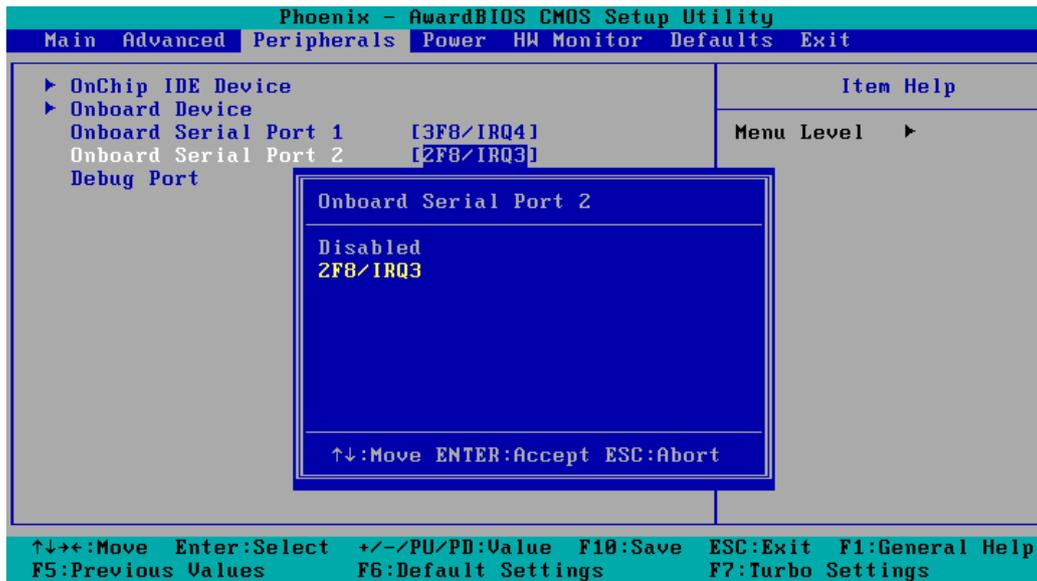
This function allows you to enable/disable serial port 2 communication. The V2101 computer will automatically distribute the IRQ value for serial port 2 as the default value. If you wish to disable, select **Disabled**.
