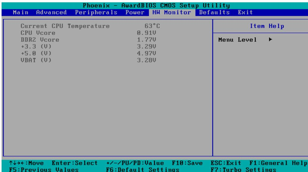
This item helps monitor the status of the system, including CPU temperature and the voltage of the CPU, SDRAM and battery.
