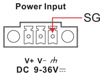
**SG:** The **Shielded Ground** (sometimes called Protected Ground) contact is the rightmost of the 3-pin power terminal block connector, when viewed from the angle shown here. Connect the SG wire to an appropriate grounded metal surface.
