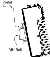
**STEP 2:** The DIN-Rail attachment unit will snap into place as shown below.
