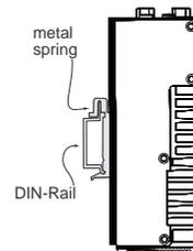
To remove the V2101 from the DIN-Rail, simply reverse Steps 1 and 2.
