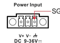
**SG:** The Shielded Ground (sometimes called Protected Ground) contact is the right most of the 3-pin power terminal block connector when viewed from the angle shown here. Connect the SG wire to an appropriate grounded metal surface.
