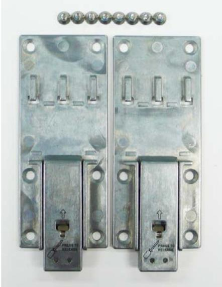
To attach the DIN-rail kit, turn the V2401/2402 over to the bottom cover. Find the locations for the screws and place the brackets on the cover. Please note that all eight screws must be firmly attached so that the computer can be securely installed on the DIN-rail.
