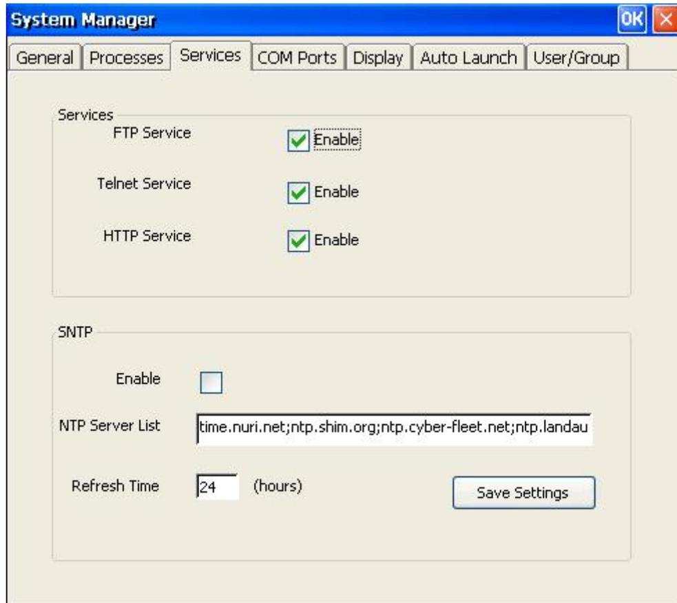
You can also adjust the time automatically by using SNTP. Select the checkbox to enable the service and then click the button next to the checkbox to activate it.
