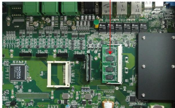
4. To upgrade the memory, you need to remove the original memory by pushing two clutches at both sides of the module.
