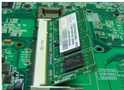
6. Push the memory all the way down to complete installation.
