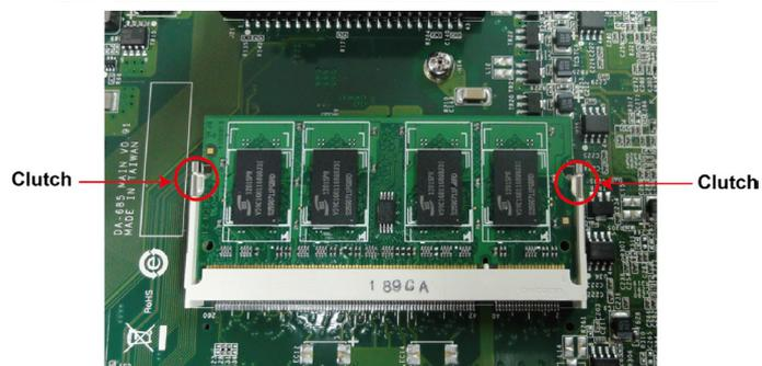
5. Gently insert the new memory into the module. Make sure the direction is correct.
