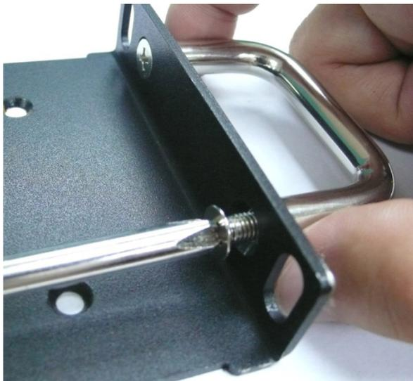
**Step 3: Installing the rack ears to the DA-685**
