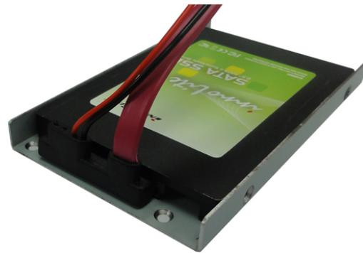
5. Place the drive bracket into the mounting space; fasten the bracket to the case using four screws, one on each corner
