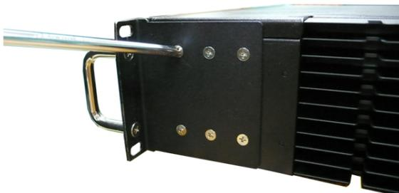
**Step 4: Installing the DA-685 to a rack**
