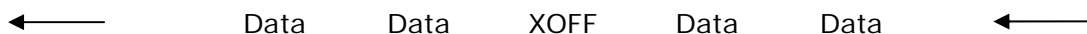
Fig. 4: Including XOFF in the data stream could result in too much of a delay.
