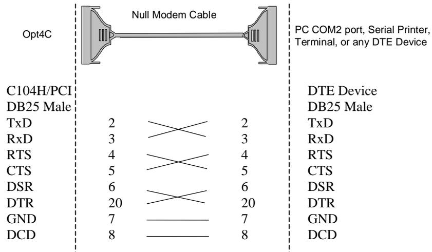
Connection Cable and Cable Wiring
