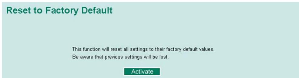
This function provides users with a quick way of restoring the IKS-6500's configuration to factory defaults. This function is available in the serial, Telnet, and web consoles.
