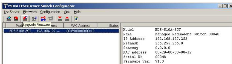
3. Click the **Upgrade Firmware** toolbar icon
