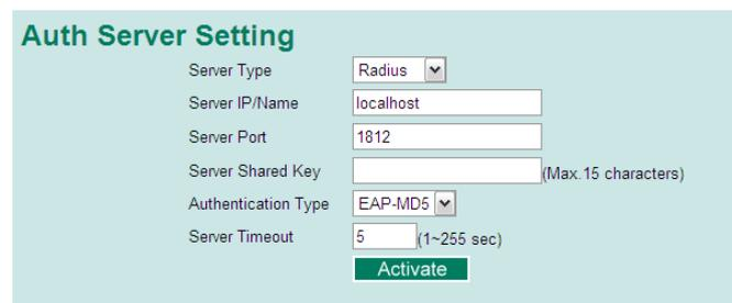
The screenshot shows the 'Auth Server Setting' interface for RADIUS. The 'Server Type' is set to 'Radius'. Other fields include 'Server IP/Name' (localhost), 'Server Port' (1812), 'Server Shared Key' (empty, with a note '(Max. 15 characters)'), 'Authentication Type' (EAP-MD5), and 'Server Timeout' (5, with a note '(1~255 sec)'). A green 'Activate' button is at the bottom.
