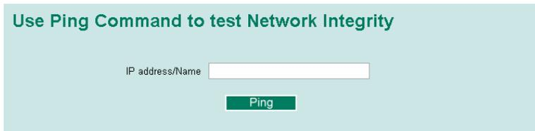
The **Ping** function uses the *ping* command to give users a simple but powerful tool for troubleshooting network problems. The function’s most unique feature is that even though the ping command is entered from the user’s PC keyboard, the actual ping command originates from the Moxa switch itself. In this way, the user can essentially sit on top of the Moxa switch and send ping commands out through its ports.
