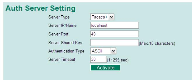
The screenshot shows the 'Auth Server Setting' interface for TACACS+. The 'Server Type' is set to 'Tacacs+'. Other fields include 'Server IP/Name' (localhost), 'Server Port' (49), 'Server Shared Key' (empty, with a note '(Max. 15 characters)'), 'Authentication Type' (ASCII), and 'Server Timeout' (30, with a note '(1~255 sec)'). A green 'Activate' button is at the bottom.
