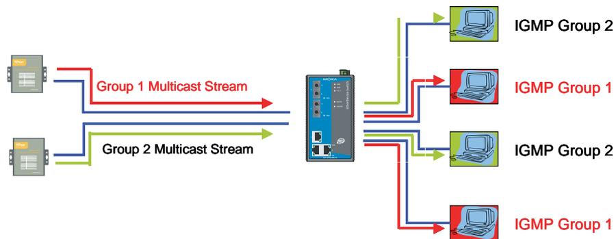
**NOTE** The VPort 251 is the source that delivers the multicast video stream. To benefit from the Multicast protocol, the gateway or network switch should support the multicast filtering function (such as IGMP Snooping) so that the multicast stream is delivered correctly and precisely. To learn more about IGMP Snooping, refer to the Moxa EtherDevice™ series Industrial Ethernet Switch user's manual.
