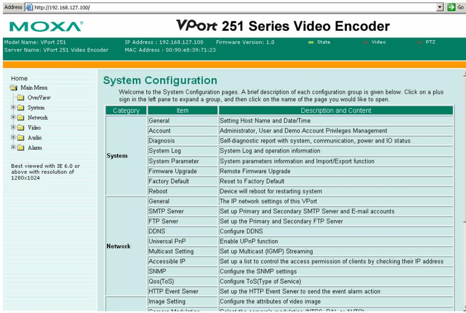
**NOTE** In the web console, administrators may navigate to **System Configuration → System → Account** to set up an administrator's password for authentication purposes. The administrator account name is admin. When a password has been set up, an authentication window will appear whenever someone attempts to open the unit's web console.
