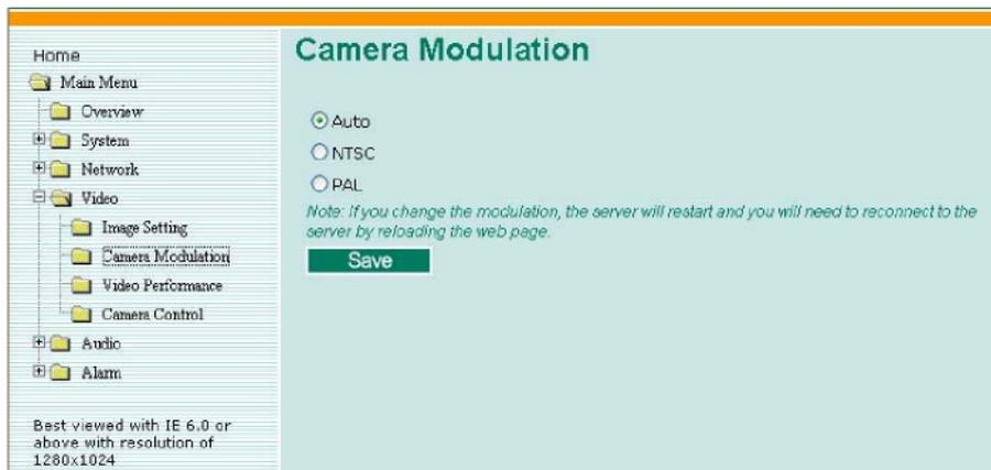
**NOTE** Changing the modulation requires resetting the server to detect the camera. Please ensure that your configurations are saved before resetting the server.
