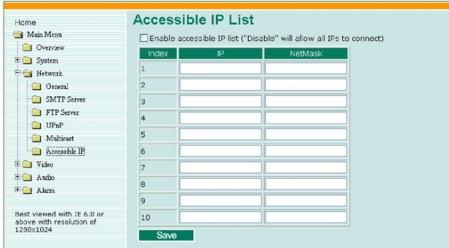
Accessible IP Settings allow you to add or remove “Legal” remote host IP addresses to prevent unauthorized access. Access to the VPort is controlled by IP address. That is, if a host’s IP address is in the accessible IP table, then the host will be allowed access to the VPort. Administrators can allow one of the following cases by setting this parameter:
