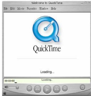
**Step 2:** When the following pop-up window appears, type the URL in the input box. E.g., type **rtsp://<VPort 251's IP address>[:<RTSP Port>]/unicaststream**
