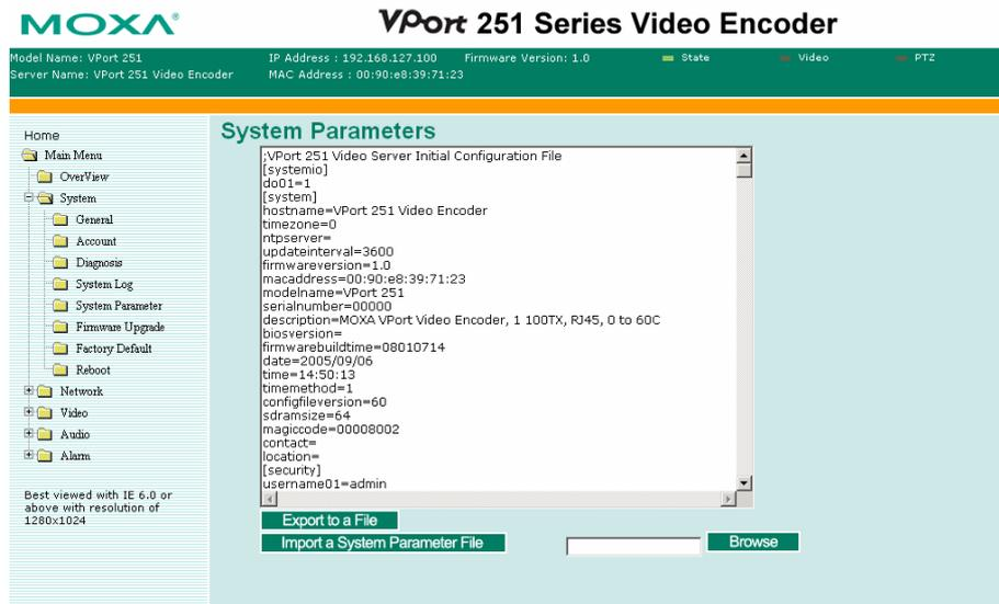
**NOTE** The system parameter import/export functions allow the administrator to backup and restore system configurations. The Administrator can export this sys\_config.ini file (in a special binary format) for backup, and import the sys\_config.ini file to restore the system configurations of VPort video encoders. System configurations will be changed immediately after the VPort is rebooted.
