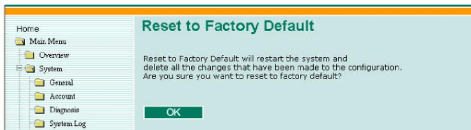
**NOTE** All parameters will be reset to factory defaults when you use the **Factory Default** function. For this reason, if you want to keep a digital copy of the current configuration, remember to export the sys\_config.ini file before using the Factory Default function.
