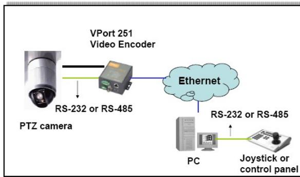
**NOTE** The PTZ control panel or keyboard must support the control of PTZ camera being used.
