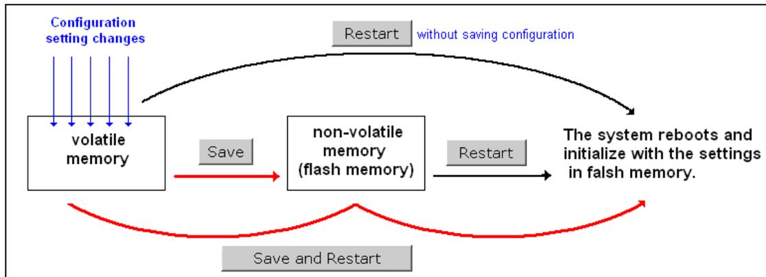
After you click on **Save Configuration** in the left menu box, the following screen is displayed. Click **Save** if you wish to update the configuration settings in the flash memory at this time. Alternatively, you may choose to run other functions and put off saving the configuration until later. However, the new setting changes will remain in the non-volatile memory until you save the configurations.
