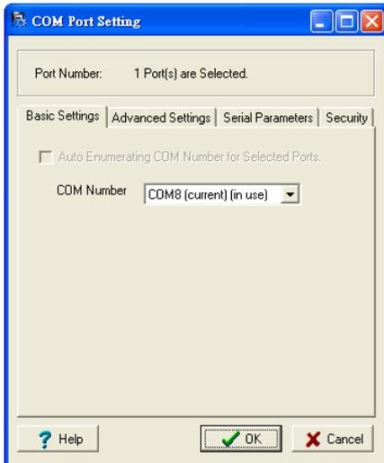
8. Click the **Advanced Setting** tab to modify Tx Mode, FIFO, Fast Flush, and other parameters.
