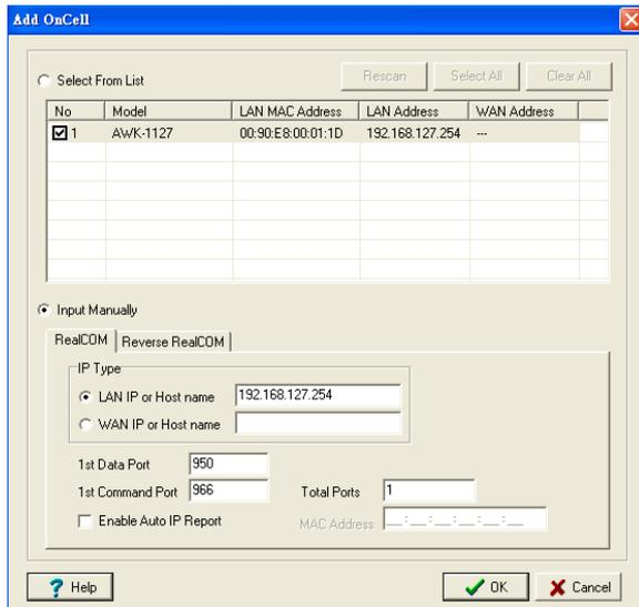
4. COM ports and their mappings are displayed in blue until they are activated. Activating the COM ports saves the information in the host system registry and makes the COM port available for use. The host computer will not have the ability to use the COM port until the COM ports are activated. Click **Yes** to activate the COM ports at this time, or click **Cancel** to activate the COM ports later.
