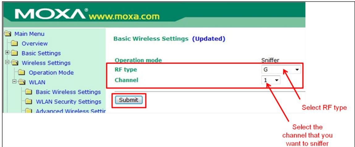
On a computer connected to the AWK, you can use a packet analyzer to view network traffic on an interface. The following steps describe how to configure Wireshark to analyze packets on the AWK.
