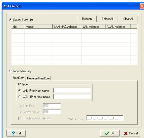
Alternatively, for RealCOM mode, you can select **Input Manually** and then manually enter the AWK-1127 's IP Type. To do this, select LAN type, followed by **1st Data Port**, and **1st Command Port** for the COM ports that will be mapped to. Click **OK** to proceed to the next step. Note that the **Add OnCell** page supports FQDN (Fully Qualified Domain Name), in which case the IP address will be filled in automatically.
