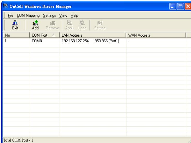
7. Click on the created COM port to select it. Then right click to select Basic Setting tab. On the **Basic Setting** tab, use the **COM Number** drop-down list to select a COM number to be assigned to the AWK-1127’s serial port that is being configured. Note that ports that are “in use” will be labeled accordingly.
