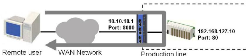
**NOTE** Make sure that the AWK is operating in Client-Router mode and that the NAT function is enabled.
