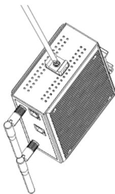
**STEP 1:** Screw the cable holder onto the bottom of the AWK-3121-M12.
