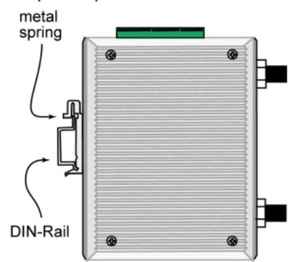
To remove the AWK-3121-M12 from the DIN-Rail, simply reverse Steps 1 and 2.
