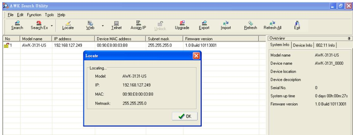
5. Make sure your AWK is **unlocked** before using the search utility's icons setting. The AWK will unlock automatically if the password is set to the default. Otherwise you must enter the new password manually.
