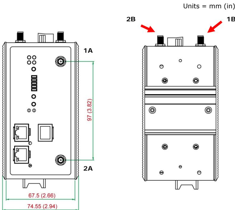
The AWK-5232 provides dual RF technology that meets the 802.11 a/b/g/n standards, giving full 2x2 MIMO. Antennas 1A and 1B are the MIMO antennas associated with RF1, and 2A and 2B are the MIMO antennas associated with RF2.
