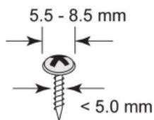
Do not screw the screws all the way in to the wall—leave a space of about 2 mm to allow room to slide the wall-mounting kit between the wall and the screws.
