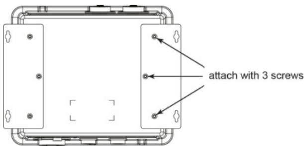
**STEP 2:** Mounting the TAP-6226 on the wall requires 4 screws. Use the TAP-6226 device, with wall-mounting kit attached, as a guide to mark the correct locations of the 4 screws. The heads of the screws should be between **5.5 mm** and **8.5 mm** in diameter, and the shafts should not be more than 5.0 mm in diameter, as shown in the figure.
