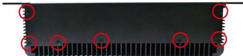
4. Remove the back cover of the computer. You will see two HDD brackets inside. The memory module is located below the first HDD bracket.
