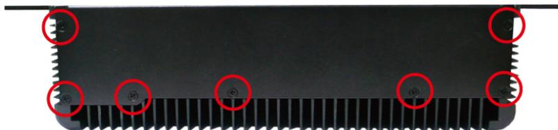
5. Remove the back cover of the computer. You will see two HDD brackets inside. The memory module is located below the first HDD bracket.
