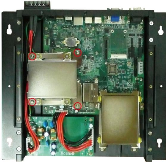
2. Remove two black screws on each side of the bracket, and then take off the cover.
