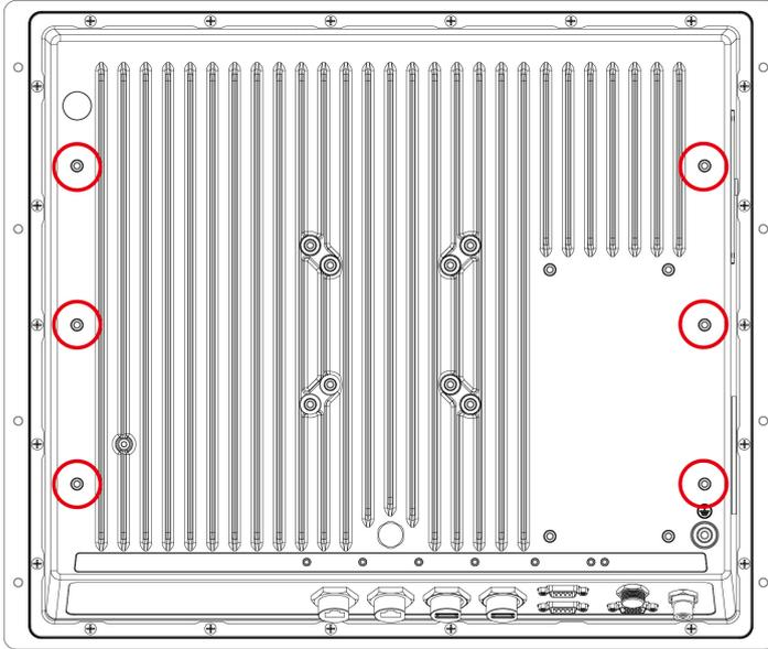
**NOTE** To make sure the panel computer will be securely installed on the yoke, use **M4** screws. The screw holes penetrate 8 mm into the computer's case. When choosing screws for installation, remember to account for the thickness of the mounting surface. Refer to [Appendix B: Statement of Regulatory Approval](#) for the technical details regarding regulation Class 1 Div. 2 devices.
