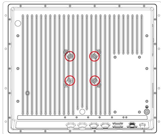
**NOTE** To make sure the panel computer will be securely installed on a wall, we suggest you to use the screws with the specifications of **M4**. The screw holes penetrate 6 mm into the computer's case. When choosing screws for installation, remember to account for the thickness of the mounting surface. Refer to **Appendix B: Statement of Regulatory Approval** for the technical details regarding regulation Class 1 Div. 2 devices.
