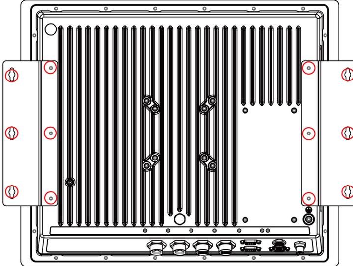
**NOTE** To make sure the panel computer will be securely installed on a wall, we suggest you to use **M5** screws of a suitable length to guarantee the computer remains securely fastened to the mounting point. The screw holes penetrate 8 mm into the computer's case. When choosing screws for installation, remember to account for the thickness of the mounting surface.
