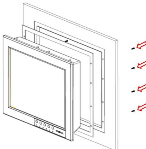
**NOTE** To make sure the panel computer will remain securely installed in the cabinet, use **M6** screws of a suitable length. The screw holes penetrate 6 mm into the computer's case. When choosing screws for installation, remember to account for the thickness of the mounting surface.
