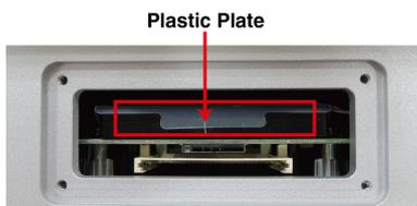
3. Remove the screws on two sides of the SSD, and then remove the plastic plate.
