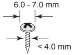
Do not screw the screws in all the way—leave a space of about 2 mm to allow room for sliding the ToughNet switch between the wall and the screws.
