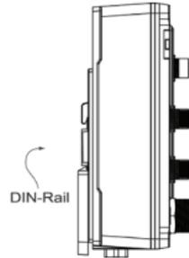
To remove the Moxa ToughNet Switch from the DIN-Rail, use a screwdriver to pull down the bottom parts of the two spring-loaded brackets until they are fixed in the "locked" position, and then reverse Steps 3 and 4 above.
