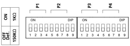
Each port consists of 4 pins; you must switch all 4 pins of a port simultaneously to adjust the value of the port.
