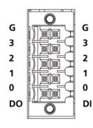
The UC-5100 Series comes with 4 digital inputs and 4 digital outputs. The DI/DO connectors are located on the top panel of the computer. Refer to the diagram on the left for the pin definitions. For the wiring method, refer to the following figure:
