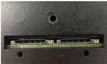
2. Insert the Micro SIM-card into the socket in the correct direction.
