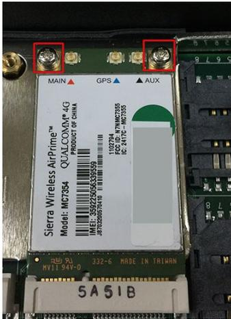
3. Attach the flat end of the antenna cable to the connector marked MAIN on the module. Follow the procedure described above to attach the AUX antenna cable. If your UC-8540 is not a standalone GPS version, you can attach the GPS antenna cable to the connector marked GPS on the module.
