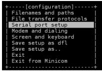
4. Select **A** to change the serial device. Note that you need to know which device node is connected to the ioThinx 4530 controller.
