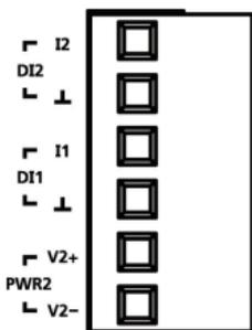
VPort 461A has two sets of digital inputs, DI1 and DI2. Each DI consists of two contacts of the 6-pin terminal block connector, on the VPort's top panel. Top view of one of the terminal block connectors is shown here.
