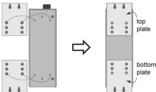
**Step 2:** Mounting VPort 461A on the wall requires 4 screws. Use the VPort 461A, with wall mount plates attached, as a guide to mark the correct locations of the 4 screws. The heads of the screws should be less than 6.0 mm in diameter, and the shafts should be less than 3.5 mm in diameter, as shown in the figure on the right.
