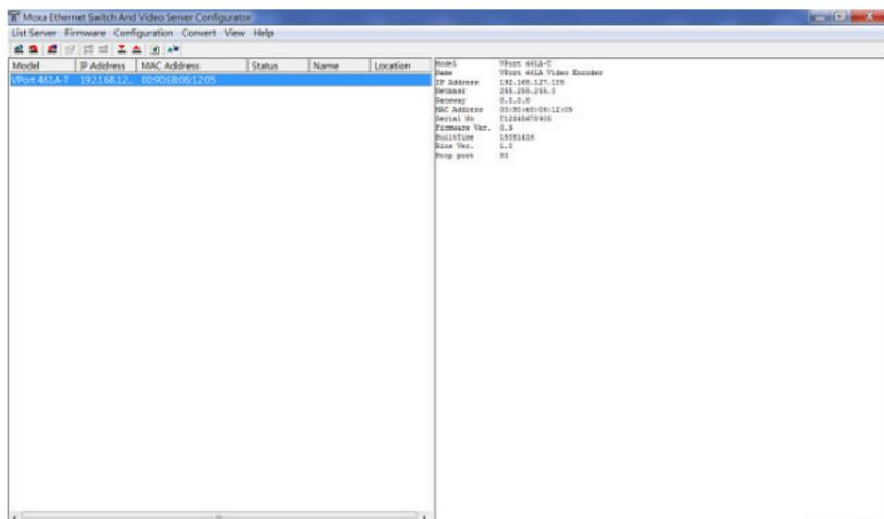
**NOTE** Broadcast Search can only search for devices connected to the same LAN subnet as the VPort. If your devices are located on a different LAN subnet, use the "Specify IP Address" function to search for the device by keying in the IP address.
