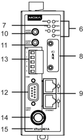
11. AUDIO INPUT port for mic-in and line-in connection
