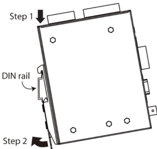
To remove the VPort 461A from the DIN-Rail, do the following:
