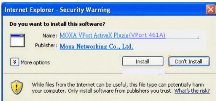
**NOTE** For Windows XP SP2 or later operating systems, the ActiveX Control component will be blocked for system security reasons. In this case, the VPort's security warning message window may not appear. Users should unblock the ActiveX control function or disable the security configuration to enable the installation of VPort's ActiveX Control component.
