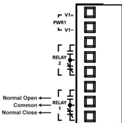
The VPort 461A has two sets of relay output, relay 1 and relay 2, which are located on the 8-pin terminal block connector. Each relay output consists of the 3 contacts of the terminal block on the VPort 461A's top panel.
