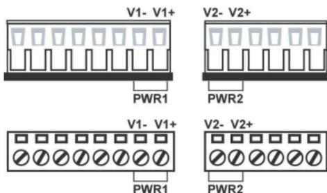
The VPort 461A has two sets of power inputs, power input 1 and power input 2, which are located on the 6-pin and 8-pin terminal block connectors. Top and front views of the terminal block connectors are shown here.
