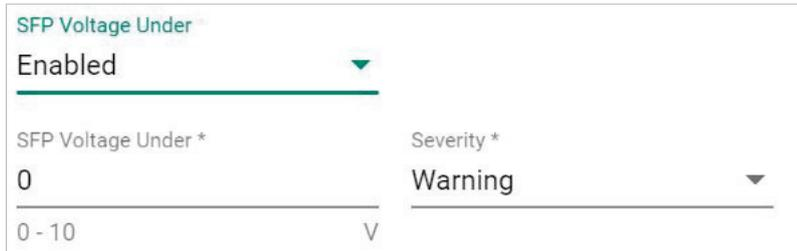
The screenshot shows a configuration form for 'SFP Voltage Under'. The first dropdown menu is set to 'Enabled'. Below it, the 'SFP Voltage Under \*' field has a value of '0' and a unit of 'V' with a range of '0 - 10'. To the right, the 'Severity \*' dropdown menu is set to 'Warning'.
