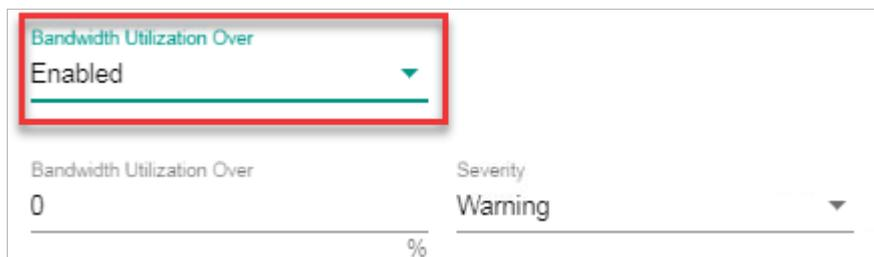
The screenshot shows a configuration screen for 'Bandwidth Utilization Over'. The first dropdown menu, labeled 'Bandwidth Utilization Over', is highlighted with a red box and shows 'Enabled' selected. Below it, there is a numerical input field for the threshold, currently set to '0', followed by a '%' symbol. To the right of the threshold field is a 'Severity' dropdown menu, currently set to 'Warning'.
