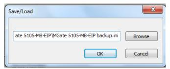
Wait for the MGate Manager to finish configuring the target device. If you import the configuration file successfully, a confirmation message will pop up. After closing the message dialog, the MGate Manager will automatically execute a Broadcast Search for all MGate units on the LAN. Your MGate should reappear in the list of units.
