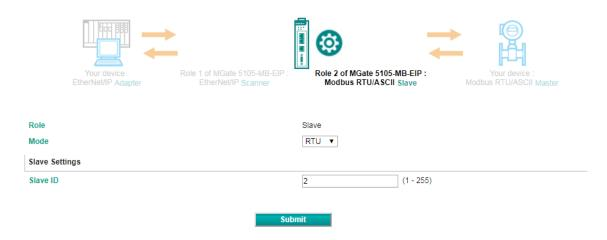
In RTU/ASCII Master mode, the MGate works as a Modbus client/master device and will send the Modbus request to the Modbus network actively.
