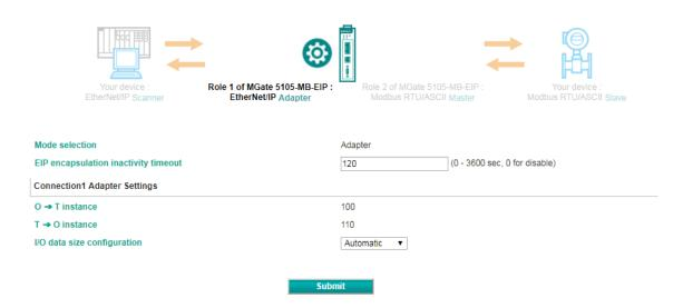
If you select EtherNet/IP Adapter as your device, the MGate 5105-MB-EIP will be configured as Ethernet/IP Scanner. In Scanner mode, you must designate the parameters for each connection. Refer to your EtherNet/IP adapter's datasheet to fill out O(T and T(O parameters.
