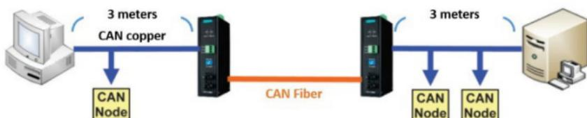
The maximum length for CAN fiber is 2 km (depending on the data rate and the protocol used). This table below suggests the maximum fiber lengths at certain baud rates as per ISO-11989-2 while using no more than 3m of the CAN Bus cable in the CAN bus network.
