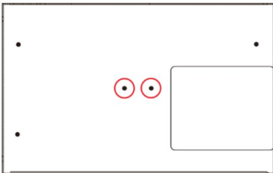
Place the black plate and fasten with two screws.
