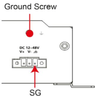
**SG:** The Shielded Ground (sometimes called Protected Ground) contact is the right most contact on the 3-pin power terminal block connector when viewed from the angle shown here. Connect the SG wire to an appropriate grounded metal surface. An additional ground connector is provided just above the power terminal block, which you can use for grounding protection.
