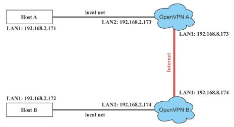
The configuration procedure is almost the same as for the previous example. The only difference is that you will need to comment out the parameter up in /etc/openvpn/tap0-br.conf of OpenVPN A and /etc/openvpn/tap0-br.conf of OpenVPN B.
