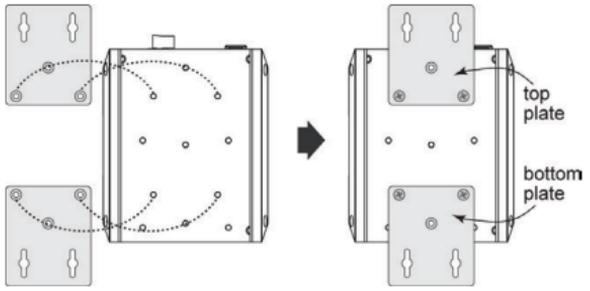
**STEP 2:** Mounting the EDS-528E series on a wall requires 4 screws. Use the EDS-528E, with wall mount plates attached, as a guide to mark the correct locations of the 4 screws. The heads of the screws should be less than 6.0 mm in diameter, and the shafts should be less than 3.5 mm in diameter, as shown in the figure on at the right.
