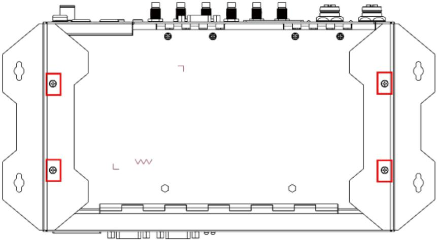
The four screws for the mounting brackets are included in the product package. They are standard IMS\_M3x5L screws and require a torque of 4.5 kgf-cm. Refer to the following illustration for details.
