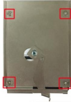
4. Unfasten the screw on the storage slot cover and slide the cover down to access the slot.
