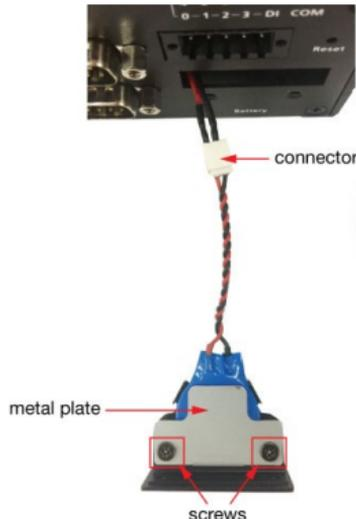
4. Separate the connector and remove the two screws on the metal plate.
