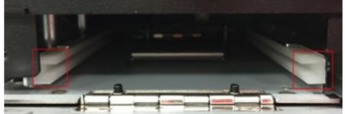
6. Insert the tray so that it aligns with the rails on both sides and slide the tray into the slot.
