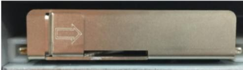
To take out the tray, simply pull the clutch to the right and pull the tray out.
