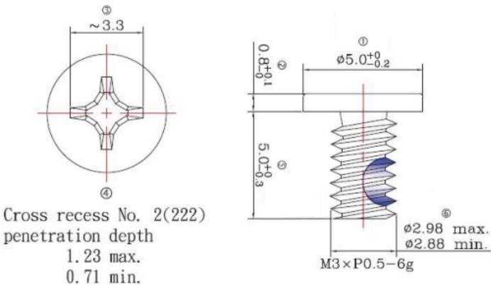
Use two screws (M3\*5L standard is recommended) on each side to attach the V2406C to a wall or cabinet. The product package does not include the four screws required for attaching the wall-mounting kit to the wall; they need to be purchased separately. Ensure that the V2406C computer is installed in the direction shown in the following figure.
