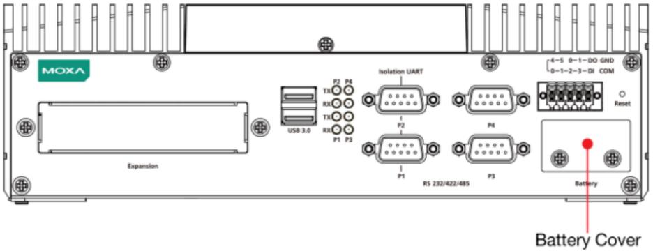
2. Unfasten the two screws on the battery cover.
