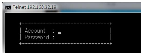
The text mode console will display the menu driven interface. Users can use arrow key to move the menu bar. To select the option, press the "Enter" key to go next level menu. To go previous level menu, press "Esc" key to quit. If necessary, MGate will need to restart to activate the setting.
