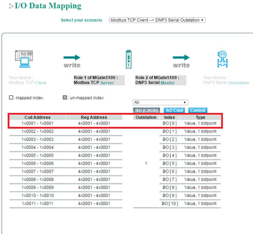
Likewise, if the Modbus master wants to read the value in DNP3 outstation index AI [0], the Modbus master must send a request to read the Modbus addresses 4x9217 and 4x9218, whose value will be periodically updated as a result of cyclic polling to the outstation on the other side.
