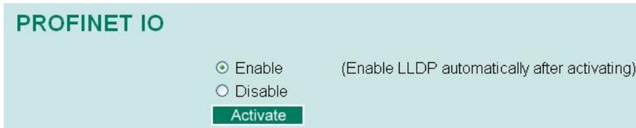
Select the **Enable** option and click **Activate** to enable PROFINET I/O. With PROFINET I/O enabled, PROFINET type LLDP will be enabled automatically.
