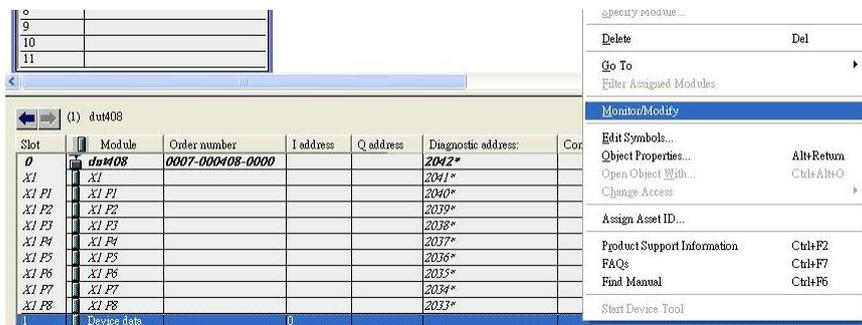
Use Monitor to check the input data value. In this dialog, you can see the status value of each address. Please refer to the **PROFINET Cyclic I/O data table** in Chapter 5.1 to see the meaning of each bit. For example, address 0.1 is Bit 1 in the **PROFINET Cyclic I/O data table**. It represents Power 1 status of the switch. 1 means Power 1 exists and **Green** will be displayed in the **Modify/monitor** window
