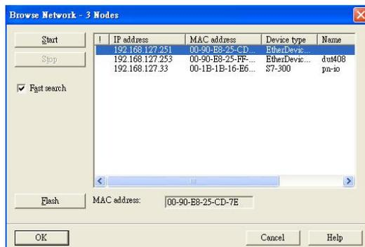
2. Assign IP address and Device name
