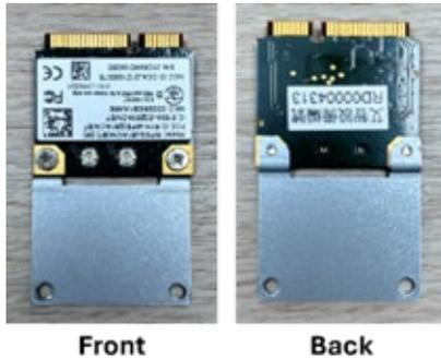
3. Insert the Wi-Fi module in the socket and use 2 M2 screws to secure the module to the socket.
