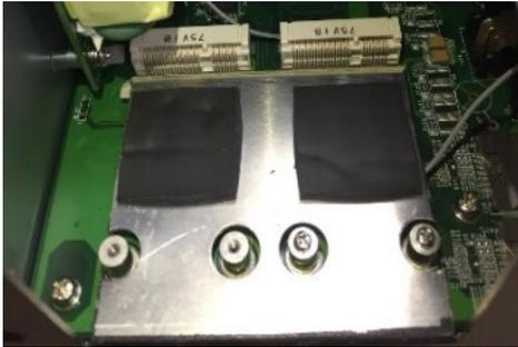
2. Insert the cellular module into the socket and tighten the two M2 screws on the module.
