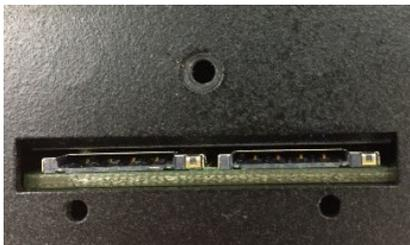
2. Push down the Micro SIM-card into the socket in the correct direction.
