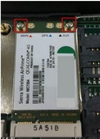
3. Attach the flat end of an antenna cable to the connector marked MAIN on the module and insert the other end of the cable into the antenna connector hole marked MAIN on the front panel of the computer.
