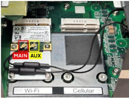
For the AUX antenna cable, use the procedure described above and remember to insert the cable into the antenna connector hole marked AUX 1 on the front panel.
