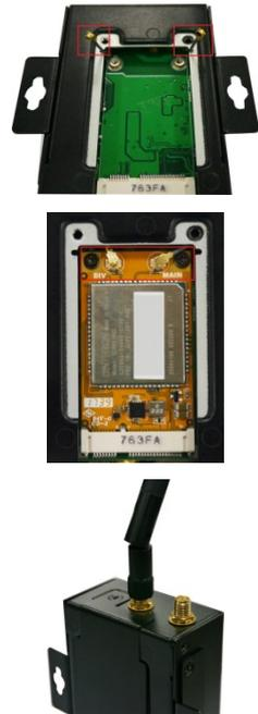
You will need the following to install a Wi-Fi module. The Wi-Fi module package consists of 1 Wi-Fi module and 2 screws. You must purchase the Wi-Fi antennas separately based on your installation requirements.
