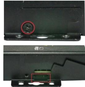
To remove the MicroSD card, push the card in and release it to allow the card to pop out.
