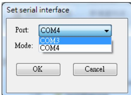
4. Select "RS232", "RS485 2 wires", or "RS422/RS485 4 wires" from the **Mode** drop-down menu.
