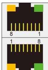
The LED indicators on the right-top (for the upper LAN connector) and right-bottom (for the lower LAN connector) corners glow a solid green color when the cable is properly connected to a 100 Mbps Ethernet network. The LED will flash on and off when Ethernet packets are being transmitted or received.
