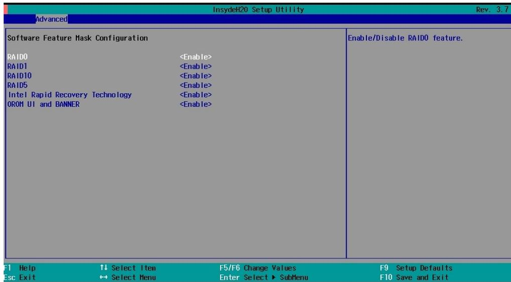
**RAID 0** is a simple striping of information across two drives. It offers marginal improvements in access times for substantial sacrifices in system reliability.
